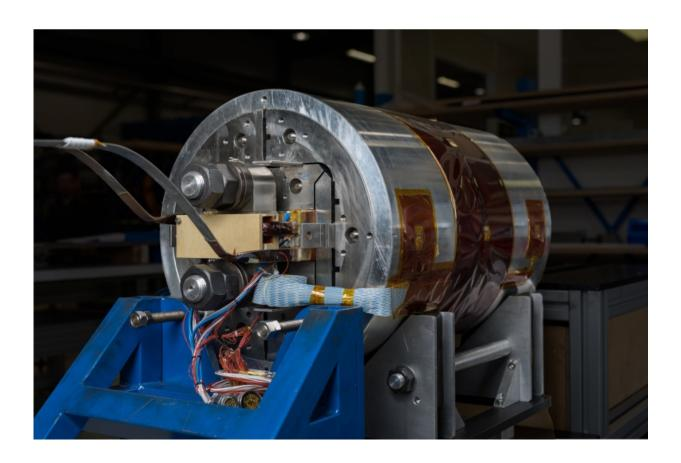
The Racetrack Model Coil test magnet Credit: CERN
