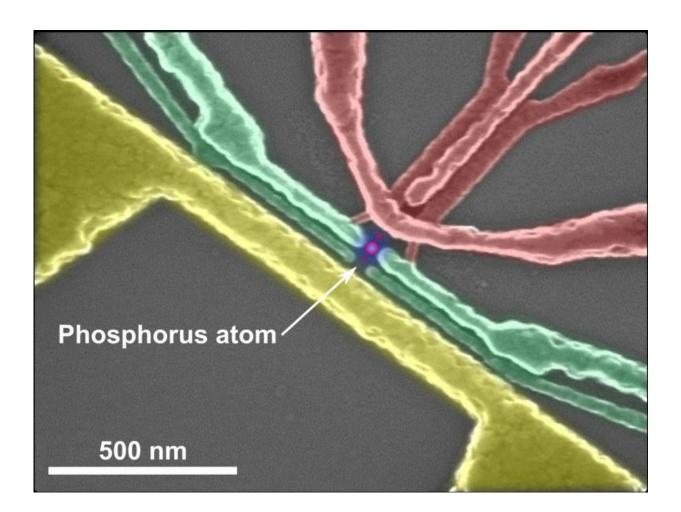
False-colour electron microscope image of the silicon nanoelectronic device which contains the phosphorus atom used for the demonstration of quantum entanglement. Credit: University of New South Wales
