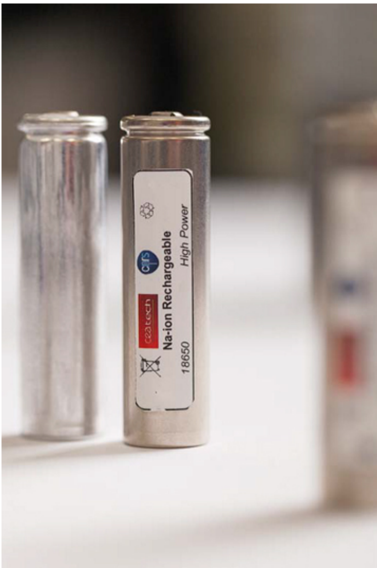
Standard "18650" sodium-ion (Na-ion) batteries, the first-ever in this format. Credit: © Vincent GUILLY/CEA
