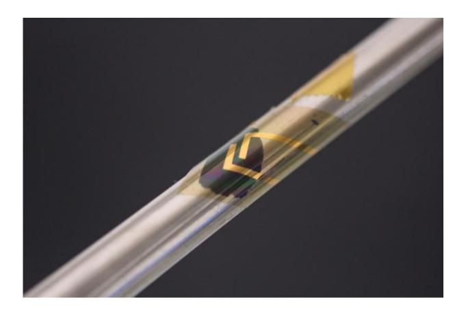
The printable sensor is thin and flexible enough to wrap around a pencil, or adapt to the form of the human body or another substrate. Device performance is largely unaffected by bending. Credit: 2015 Someya Laboratory
