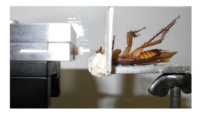
A side view onto the experimental setup wih the force sensor at the left and the specimen at the right. Credit: Tom Weihmann
