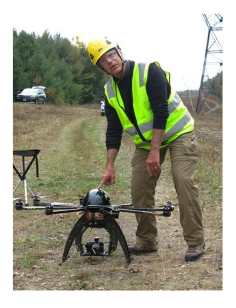
In a Wednesday, Oct. 21, 2015, photo, Bernd Lutz, CEO of Boulder, Colorado-based bizUAS Corp., which provides drone services for utilities and other industries, prepares to demonstrate the use of a Cyberhawk octocopter drone for power line inspections at a New York Power Authority site in the Catskills, near Blenheim, N.Y. Utilities plan to use drones for a range of inspection and maintenance applications to save money, improve efficiency, and increase safety for workers. (AP Photo/Mary Esch)
