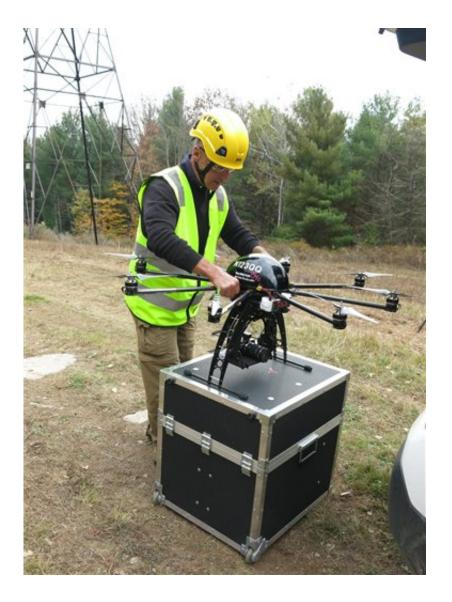
In a Wednesday, Oct. 21, 2015, photo, Bernd Lutz, CEO of Boulder, Colorado-based bizUAS Corp., which provides drone services for utilities and other industries, prepares to demonstrate the use of a Cyberhawk octocopter drone for power line inspections at a New York Power Authority site in the Catskills, near Blenheim, N.Y. Utilities plan to use drones for a range of inspection and maintenance applications to save money, improve efficiency, and increase safety for workers. (AP Photo/Mary Esch)
