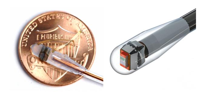
Image of the sensor encapsulated into the catheter with a US penny for scale, and (right) a photorealistic rendering of the molded system.
