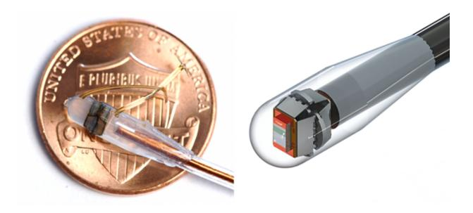
Image of the sensor encapsulated into the catheter with a US penny for scale, and (right) a photorealistic rendering of the molded system.
