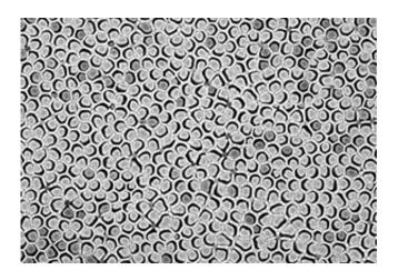
The tips of vertically aligned hollow polymer nanotubes poke out of a porous alumina template. Credit: Reproduced from Ref. 1 and licensed under CC-BY  $4.0 \odot 2014$  W. H. Liew et al.
