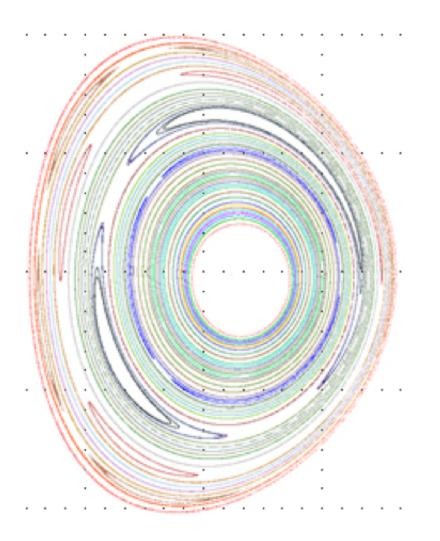
A cross-section of the virtual plasma showing where the magnetic field lines intersect the plane. The central section has field lines that rotate exactly once. Credit: Stephen Jardin
