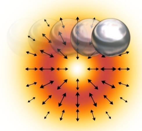
Tracked in flight: Physicists at the Max Planck Institute for the Science of Light track the path of a one-millimetre metal sphere that flies through a radially polarized laser beam in which the polarizations symbolized by arrows are arranged like the spokes of a wheel. In this kind of laser light, the polarization
