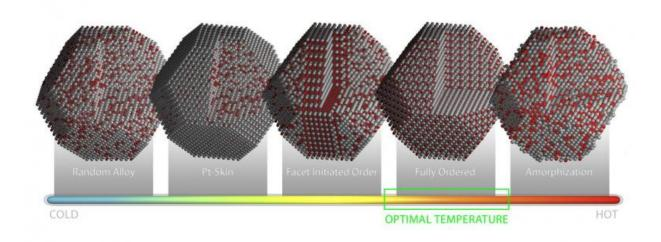
Models of platinum-cobalt nanoparticle catalysts illustrate how specific atomic configurations originate and evolve as the particles are heated. Credit: Illustration by Andy Sproles, Oak Ridge National Laboratory, US Department of Energy
