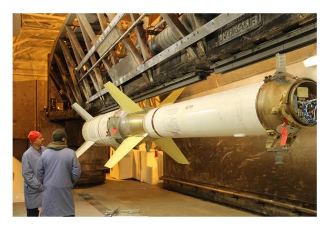
Part of CAPER, short for Cusp Alfven and Plasma Electrodynamics Rocket, is suspended from the rail that will carry the rocket out to the launch pad. CAPER's launch window will open Nov. 27, 2015, and scientists will have to wait for good weather conditions and a daytime cusp aurora before they can send their payload flying through the aurora borealis. CAPER will study the electromagnetic waves that both create the cusp aurora and send electrons flying out into space. Credit: NASA/Nate Empson
