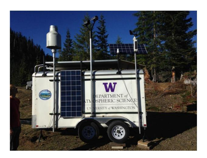
The trailer is used to mount instruments to measure rain and snow above accumulating snow pack. The instruments on the trailer operate unmanned throughout the winter season. Credit: Credits: University of Washington
