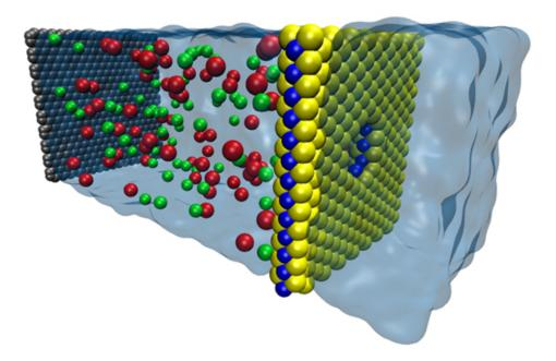
A computer model of a nanopore in a single-layer sheet of MoS2 shows that high volumes of water can pass through the pore using less pressure than standard plastic membranes. Salt water is shown on the left, fresh water on the right. Credit: Mohammad Heiranian
