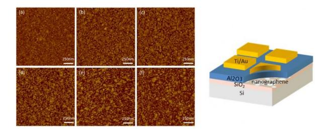
(Left) Atomic force microscope image of the nanographene film with a high density of nanographene islands, which provide more charge-trapping sites to increase store capacity. (Right) Structure of the nanographene-based charge trapping memory. Credit: Meng, et al. ©2015 IOP Publishing
