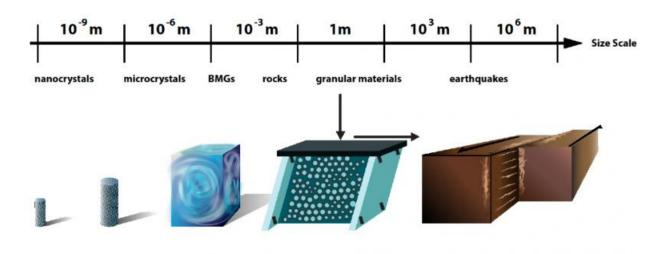
When solid materials such as nanocrystals, bulk metallic glasses, rocks, or granular materials are slowly deformed by compression or shear, they slip intermittently with slip-avalanches similar to earthquakes. Credit: University of Illinois
