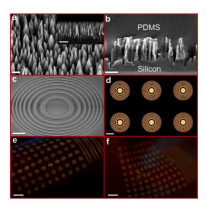
Tiny silicon nano-wire towers make up dark regions of the flexible Fresnel zone lenses. Each individual lens resembles a bulls-eye of alternating light and dark. Arrays of lenses formed within a flexible polymer bend and stretch into different
