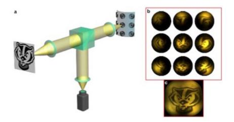
Bringing Bucky into focus. Curved arrays of individual lenses allow small-scale sensors to perceive a broader picture. The cylindrical arrangement shown in the schematic allowed researchers to resolve a 170o field of view. Credit: Hongrui Jiang
