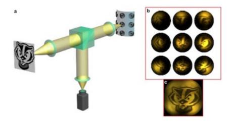
Bringing Bucky into focus. Curved arrays of individual lenses allow small-scale sensors to perceive a broader picture. The cylindrical arrangement shown in the schematic allowed researchers to resolve a 1700 field of view. Credit: Hongrui Jiang
