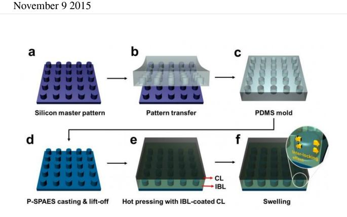
Schematic diagram of the fabrication of the pillar P-SPAES membrane and its working principle of interlocking effects. Credit: KAIST
