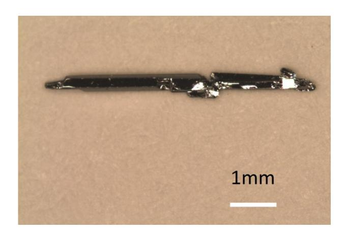
These tungsten ditelluride crystals behave as insulators for current applied in some directions and as conductors for current applied in other directions. The researchers found that this behavior is due to a newly theorized particle, the type-II Weyl fermion. Credit: Wudi Wang and N. Phuan Ong, Princeton University
