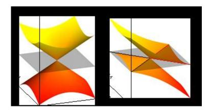
Left: Allowed states for the standard type-I Weyl fermion. When energy is tuned from below, at zero energy, a pinch in the number of allowed states guarantees the absence of many-body phenomena such as superconductivity or ordering. Right: The newly discovered type-II Weyl fermion. At zero energy, a large number of allowed states are still available. This allows for the presence of superconductivity, magnetism, and pair-density wave phenomena. Credit: B. Andrei Bernevig et al.
