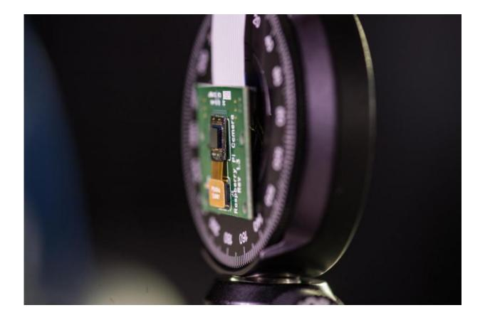
Rice University's FlatCam – the tiny chip attached to the circuit board — is a lens-less camera that may someday turn large or small surfaces into cameras. Credit: Jeff Fitlow/Rice University
