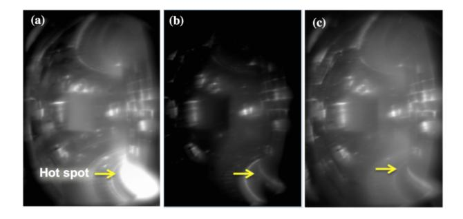
Figure 2: Infrared images of disruption heat loads on the first wall of DIII-D tokamak, when mitigated by pellets composed of (a) pure deuterium (b) mixture of deuterium and neon and (c) pure neon. Bright spots indicate high wall temperature. Primary heat loads occur where magnetic field lines intersect the wall, near bottom right of each image (hot spot indicated by arrow). Credit: C.J. Lasnier, LLNL.
