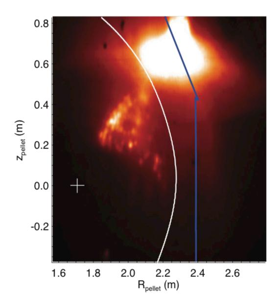
Figure 1: Visible light image of SPI into a tokamak plasma. Ice shards can be seen entering the plasma (invisible, edge indicated by white line) heading toward
