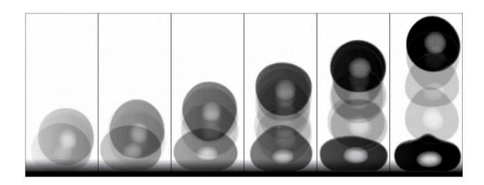
Sequential shots with a high speed camera show how the height of a bouncing water dropletincreases constantly. Credit: Tom Schutzius / ETH Zurich
