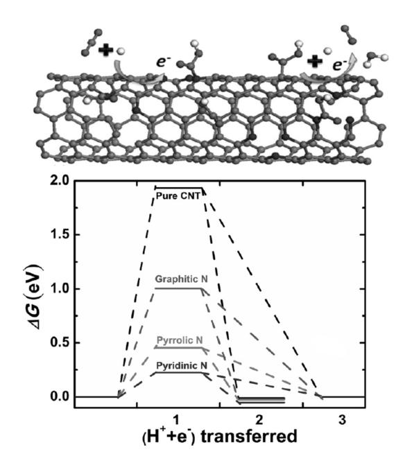
The microstructure of the nitrogen-doped carbon nanotubes was crucial to the efficiency of the catalyst. Pyridinic nitrogens within the carbon backbone were more selective for carbon dioxide reduction than pyrrolic or graphitic nitrogens. Credit: *Angewandte Chemie*
