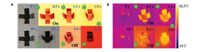
A fast self-folding box driven by light. (A) Time profiles of self-folding movements of a cross-shaped piece of paper with and without NIR light irradiation. The sample was placed on the platform and illuminated with NIR light (100 mW cm-2) normal to its surface (light is incident from above). (B) IR images of the self-folding box with and without light illumination (100 mW cm-2, NIR light). Credit: (c) 2015 *Science Advances* (2015). DOI: 10.1126/sciadv.1500533
