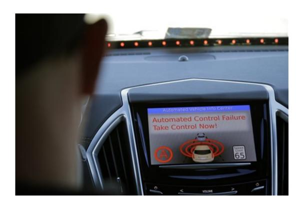
This Friday, Nov. 13, 2015, photo provided by Virginia Tech shows the Automated Vehicle Info Center display panel of a self-driving car during a test ride showing the alert system handing over control to the driver on a local street in Blacksburg, Va. (Justin Fine/Virginia Tech via AP)
