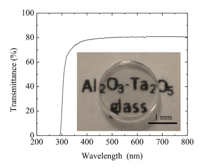
Transmittance spectrum of the 54Al2O3-46Ta2O5 glass in the UV/vis region. The inset picture shows the glass sample used for the transmittance experiment. Credit: (c) 2015 *Scientific Reports* (2015). DOI: 10.1038/srep15233
