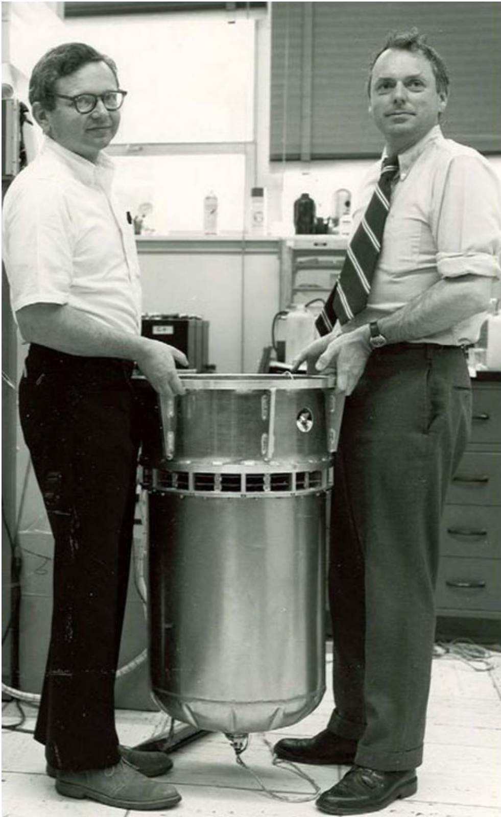
The Gravity Probe A payload of 1976, flown in a highly elliptic single orbit to measure the ‘gravitational redshift’ of Einstein’s Theory of General Relativity
