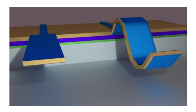
Researchers at the University of Twente's MESA+ research institute, together with researchers from several other knowledge institutions, have developed a 'flexo-electric' nanomaterial. The material has built-in mechanical tension that changes shape when you apply electrical voltage, or that generates electricity if you change its shape.
