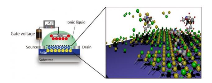
(Left) Device structure of electric-double-layer transistor with FeSe channel deposited on oxide substrate. (Right) One-monolayer FeSe is realized by electrochemical etching where Fe and Se ions are dissolved into ionic liquid. Credit: Junichi Shiogai
