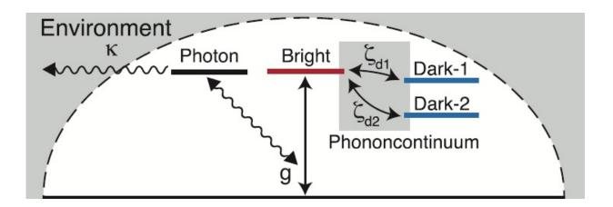
A model of energy conversion in a semiconducting carbon nanotube, showing that bright excitons are transformed into dark excitons, which have longer lifetimes and so can undergo charge separation without recombining back into photons. Credit: Yamada, et al. ©2015 American Physical Society
