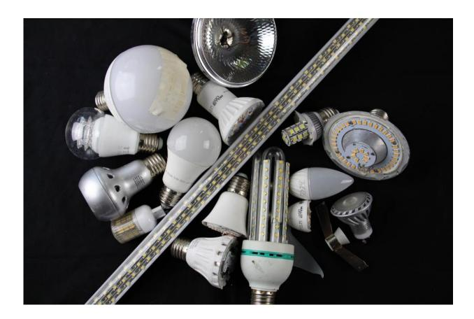
LED-based lighting elements are currently available in a variety of different forms. To recycle them efficiently they must first be broken down into their constituent parts. When recycling the LED diodes themselves it is critical that they remain as intact as possible for collection. Credit: Fraunhofer ISC/IWKS
