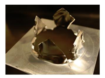
An aluminium diaphragm which is burst by gas pressure to generate a shock wave in the NPL 1.4 MPa shock tube
