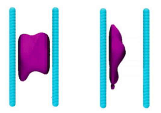
A simulated vapor tube (left) and isolated vapor cavity (right).
