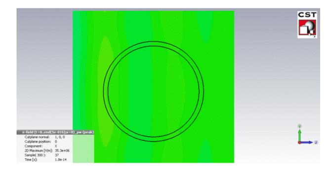
Time animation of the electric field when the meta-atom is illuminated by a light pulse. Credit: Lannebère, et al.
