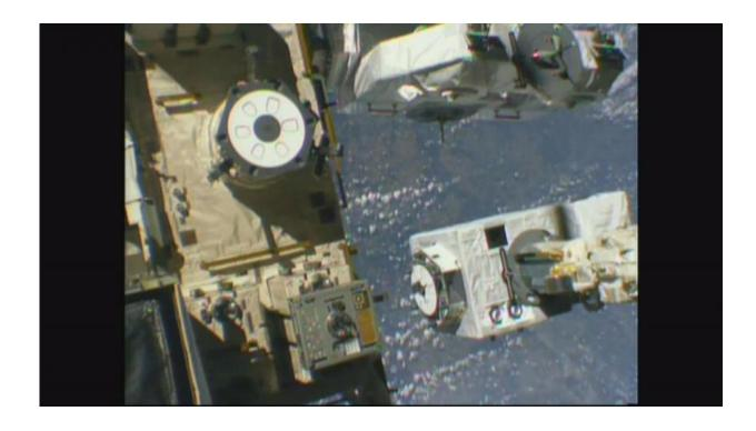
The CALorimetric Electron Telescope (CALET) is transferred from the exposed pallet to the Kibo's exposed facility. Credit: JAXA
