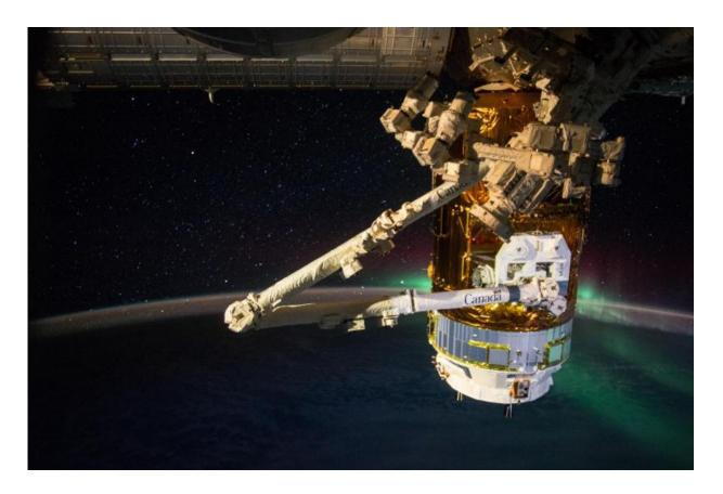
The Japan Aerospace Exploration Agency (JAXA) Kounotori H-II Transfer Vehicle (HTV-5) is seen berthed to the International Space Station. The external CALET experiment, which will search for signatures of dark matter, is seen being extracted from the unpressurized section by the station's robotic arm, Canadarm2. An aurora over the Earth limb is visible in the background. Credit: NASA
