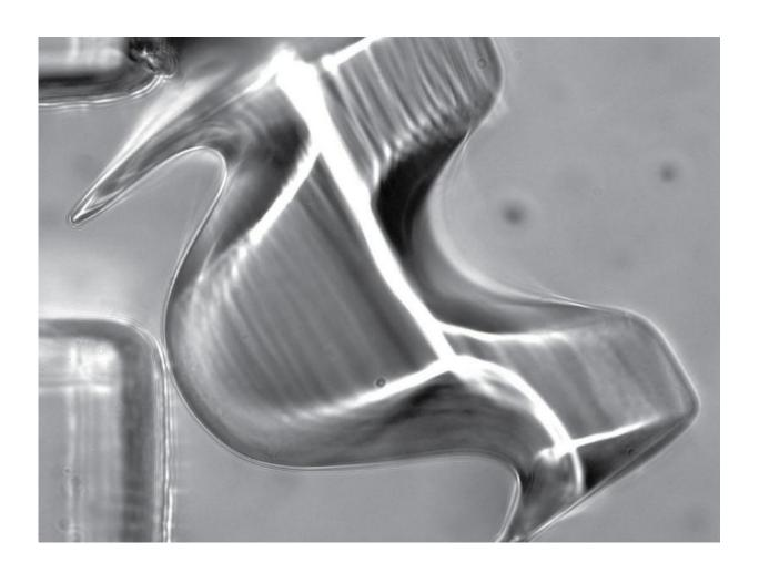
A 3-D printed microparticle about 500 micrometers in length. Credit: Chueh-Yu Wu/ UCLA
