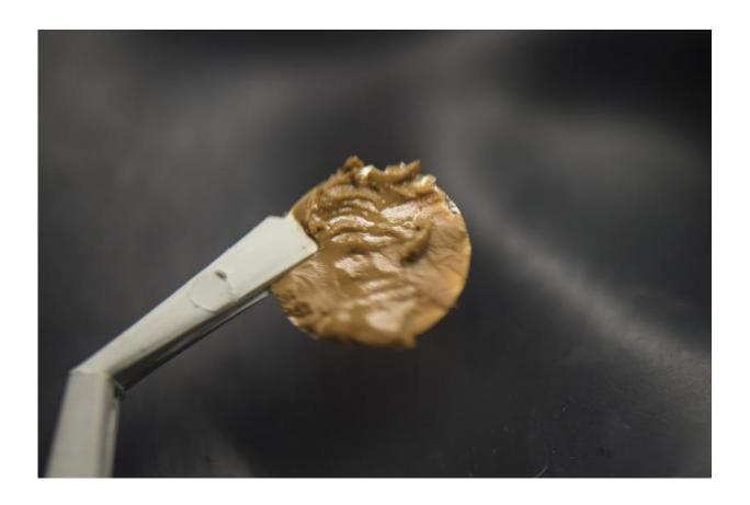
A clay-based compound invented at Rice University is an electrolyte and a separator for lithium-ion batteries for use in high-temperature environments. Credit: Jeff Fitlow/Rice University
