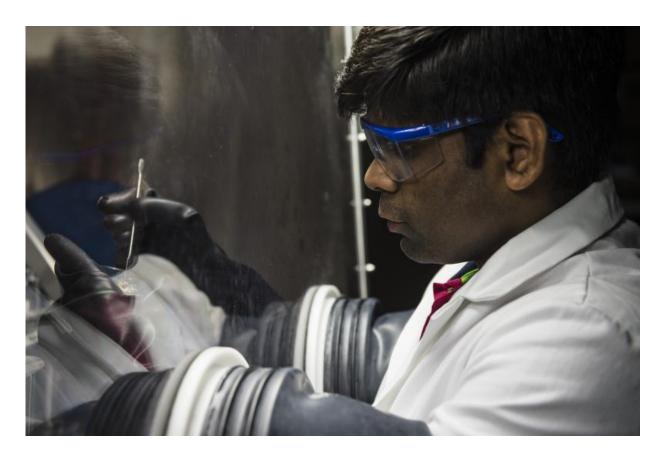
Kaushik Kalaga spreads a clay-based electrolyte/separator on one half of a button battery for testing. The batteries are meant for high-temperature environments where present lithium-ion batteries cannot be used. Credit: Jeff Fitlow/Rice University
