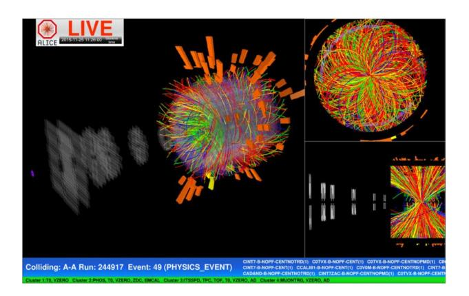
One of the very first collisions recorded between two lead ions at the LHC's top energy. The energy in the center-of-mass system is approximately 1000 TeV. Todays events bring collisions physics into a new energy scale, that of PeV (Petaelectron-volts). The ALICE detector registered tens of thousands of particles. In this live display the tracks of the particles from the collision point and through the detector are shown in colors corresponding to their mass and type. Credit: CERN
