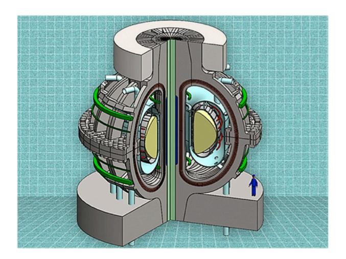
Conceptual design of the ARC fusion reactor. About the same size as the currently operating JET tokamak in the United Kingdom, but with three times the magnetic field strength, ARC is sized to produce 500 MW of deuterium-tritium fueled fusion power. Credit: Earl Marmar
