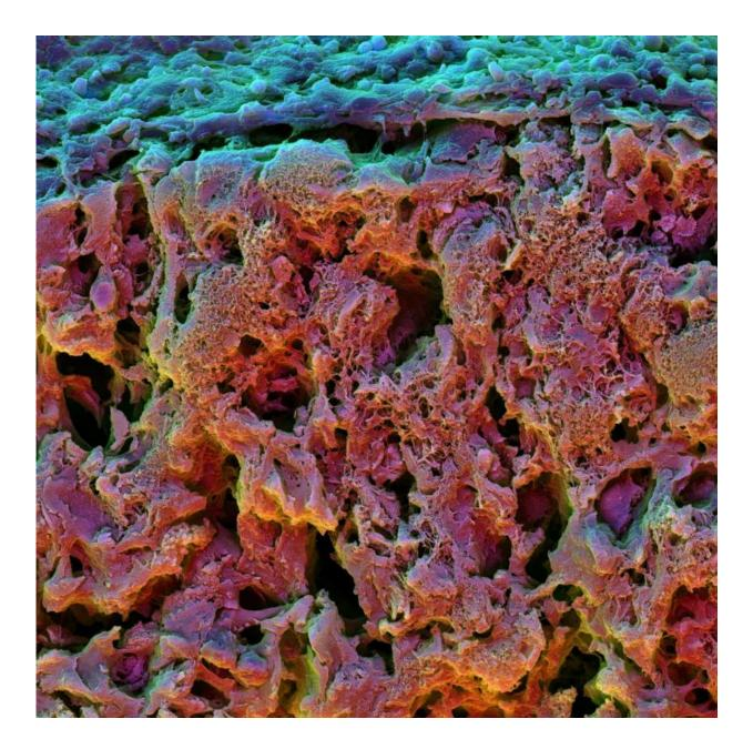
Scanning electron microscopy image of the cross section of a fast relaxing hydrogel containing mesenchymal stem cells. The cells differentiated into
