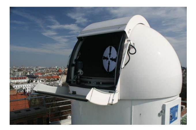
Hedy Lamarr Quantum Communication Telescope with opaque slit-mask for measuring twisted photons. Credit: University of Vienna.
