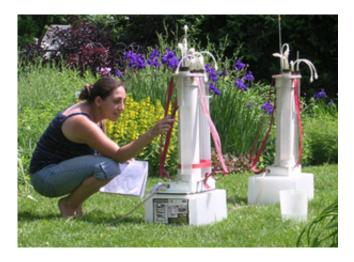
The rate of water movement through soil was measured by monitoring how quickly a hole in the ground was refilled by these unusual devices. Credit: Photo credit: M. Johnston
