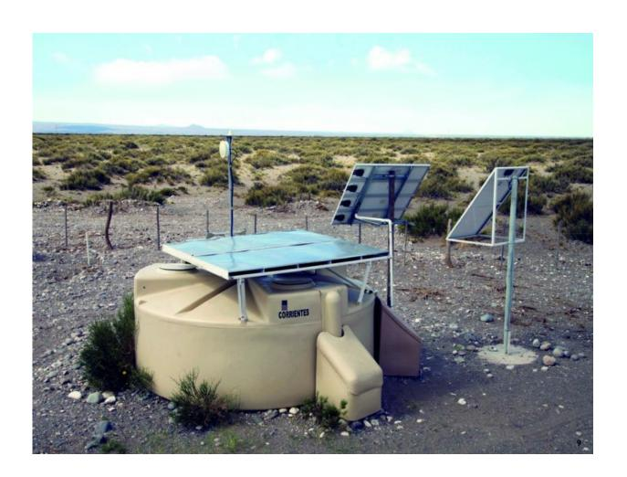
A prototype station of AugerPrime: Every water-Cherenkov detector containing 12,000 l of water is extended by a four-square-meter scintillation detector. Credit: Pierre Auger Collaboration
