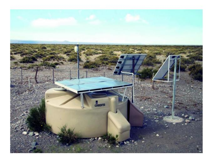
A prototype station of AugerPrime: Every water-Cherenkov detector containing 12,000 l of water is extended by a four-square-meter scintillation detector. Credit: Pierre Auger Collaboration
