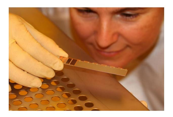
Now finished: The first, fully functional sensor module of the vertex detector in the Belle II-Experiment. Credit: L. Andricek/HLL@MPG
