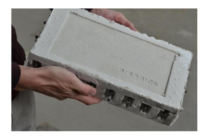
Sisbrick is a new class of earthquake-resistant building material that seismically isolates partition walls from the main building structure, significantly reducing the tension between them, thus minimizing the
