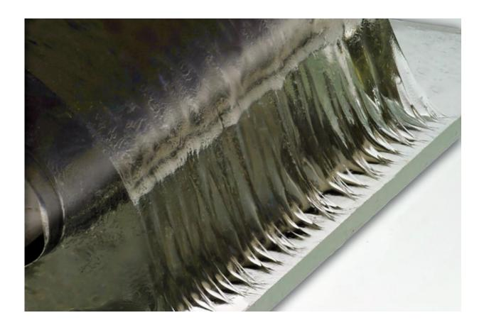
Engineered hydrogel being pulled away from a glass surface. The material shows a property called "tough wet adhesion" comparable to tendon and bone interface. The wavy edge instability at the interface is a hallmark of strongly adhered soft material on a rigid surface. Credit: Felice Frankel
