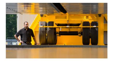
The BEAST lab simulates a decade's worth of bridge wear in less than a year. Weighted wheels shuttle across a bridge section to mimic trucks crossing 17,000 times a day. Credit: Carl Blesch
