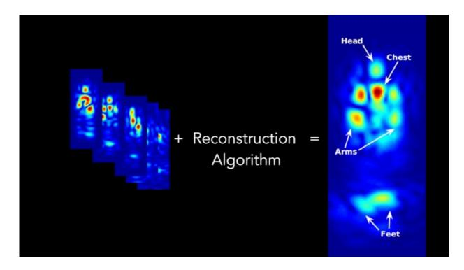
Since only a subset of body parts reflect the wireless signal back at any moment in time, the CSAIL device monitors how these reflections vary over time and stitches together a person's reflections to reconstruct his silhouette into a single image. Credit: Fadel Adib/CSAIL
