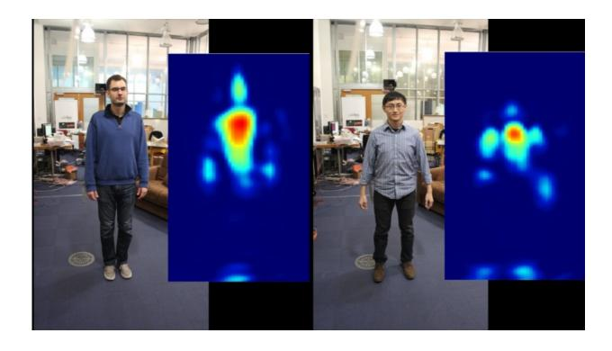
By testing different human subjects and using metrics such as height and body shape to create concrete "silhouette fingerprints" for each person, researchers can use wireless reflections to differentiate between individuals from the other side of wall. Credit: Fadel Adib/CSAIL
