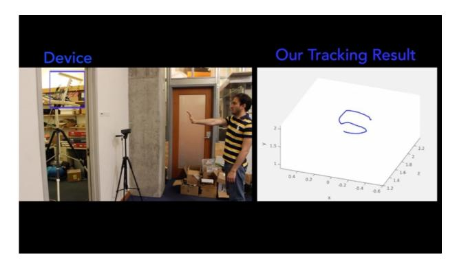
By tracking a person's silhouette, the device can trace his hand as he writes in the air. Credit: Fadel Adib/CSAIL
