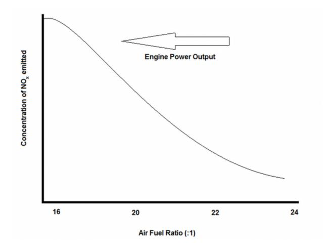
NOx emitted as a function of air fuel ratio in a diesel. Credit: Credit: BenMullins, Author provided
