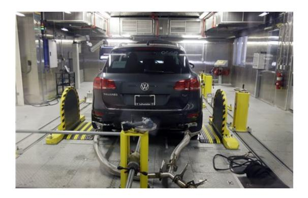
A Volkswagen Touareg diesel is tested in the Environmental Protection Agency's cold temperature test facility, Tuesday, Oct. 13, 2015, in Ann Arbor, Mich. Volkswagen has disclosed to U.S. regulators that there's additional suspect software in its 2016 diesel models that would potentially help their exhaust systems run cleaner during government tests. (AP Photo/Carlos Osorio)
